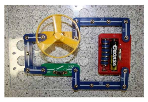
This circuit will cut the speed of the motor in half, by cutting the battery power in half. We can do this by taking out one of the batteries, and replacing it with a "short circuit" (I did this using six of the one one-snap connectors in a row). Now the fan will spin at half the speed – which is a bit safer to work with!
